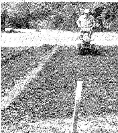
(3) Hold the handlebars with both hands and use faster tiller and engine speeds.
